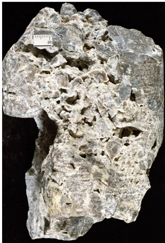
Figure 26: Brecciated dolomite core sample from 16,573 feet (5051m) [from BPC files]
